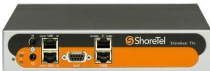
ShoreTel Voice Switches supports ShoreTel IP phones, softphones, and SIP devices. The switches will interface with standard analog trunks using loop start or wink start signaling as well as to standard analog telephones including CLASS feature phones with Caller ID Name and Number and Message Waiting. Additionally there is full support for Digital Trunks using T-1 or PRI signaling and SIP Trunking.
